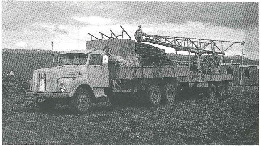
Rannsóknarbor fluttur (ljósm./photo, Birgir Jónsson). The transportation of an exploratory coring drill.
