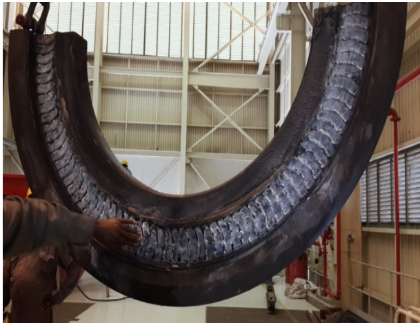
FIGURE 2: Clogged turbine nozzles
