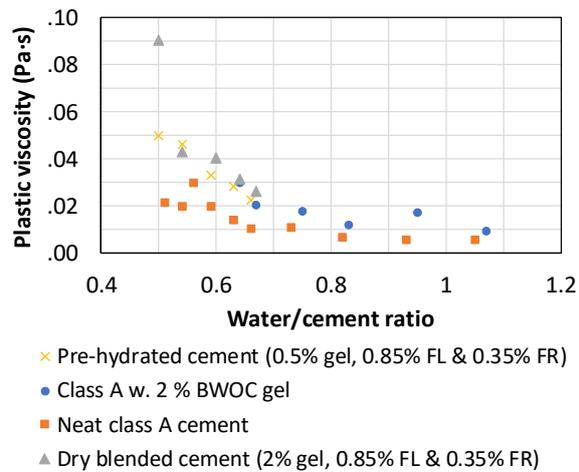
FIGURE 18: Effect of water/cement ratio on plastic viscosity
