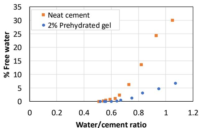
FIGURE 11: Effect of water/cement ratio on the free water in class A cement (neat) and class A cement with 2% bentonite
