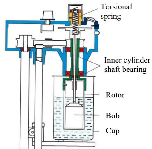
FIGURE 5: Coaxial cylinder viscometer (Nelson and Guillot, 2006)
