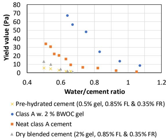
FIGURE 17: Effect of water/cement ratio on yield stress
