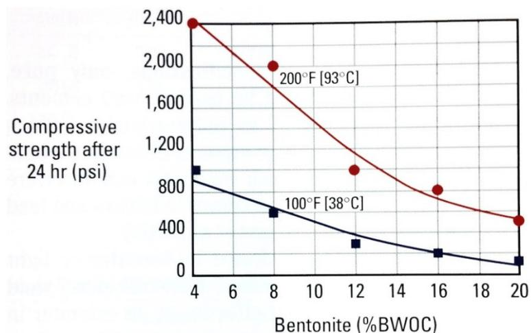
FIGURE 15: Effect of bentonite on compressive strength (Nelson and Guillot, 2006)
