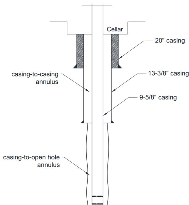
FIGURE 8: Production casing cementing
