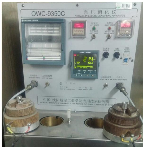
FIGURE 4: Atmospheric consistometer used by GDC
