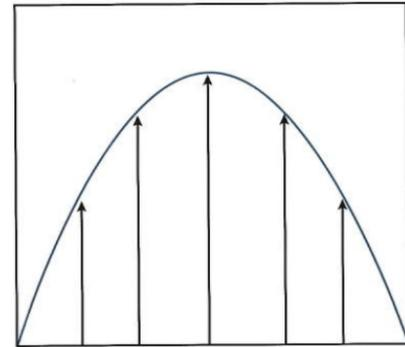
FIGURE 9: Laminar flow (Nelson and Guillot, 2006)
