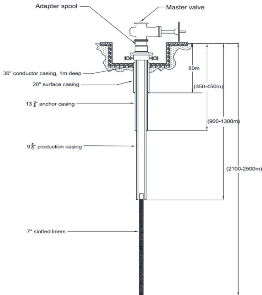
FIGURE 6: Well design for Menengai geothermal wells
