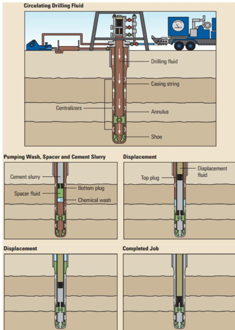
FIGURE 7: Single stage cementing process (Nelson, 2012)
