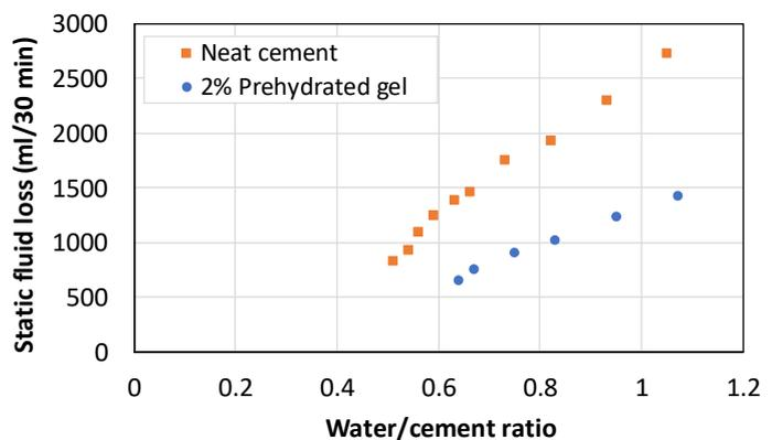
FIGURE 14: Effect of water/cement ratio on static fluid loss in class A cement (neat) and class A cement with 2% bentonite
