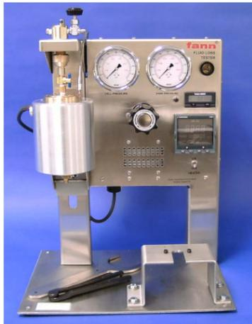
FIGURE 3: Fluid loss cell (Fann, 2014)
