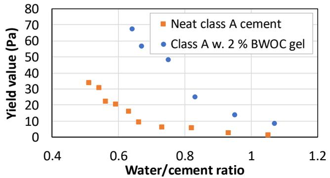
FIGURE 12: Effect of water/cement ratio on yield stress in class A cement (neat) and class A cement with 2% bentonite
