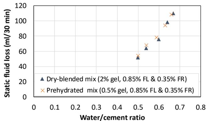
FIGURE 19: Effect of w/c on class A cement with dry blended additives and class A cement with pre-hydrated additives
