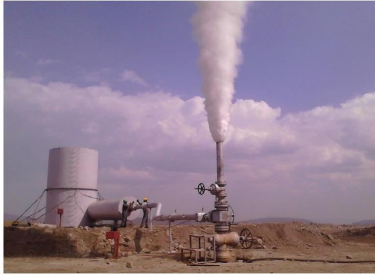
FIGURE 3: Vertical well discharge testing process with gases being released to atmosphere in Olkaria IV field, Kenya
