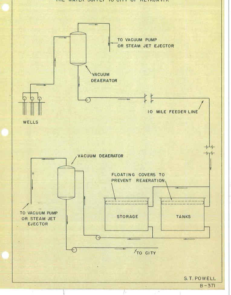
SCHEMATIC ARRANGEMENT OF EQUIPMENT FOR RECIRCULATION
