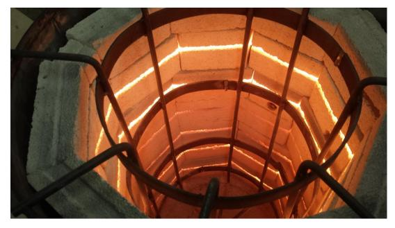
Figure 2- Heating elements for the reactor
