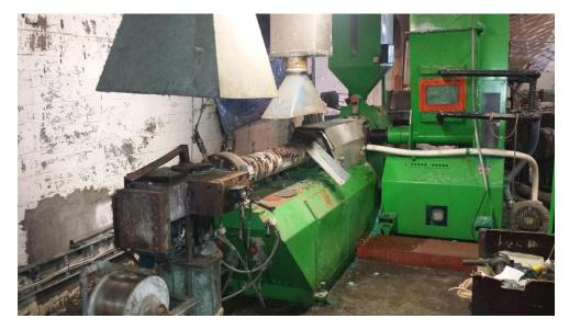
Figure 6 - Plastic extruder unit
