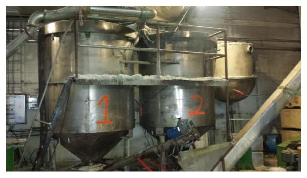
Figure 3 - Big size storage silo for shredded plastic
