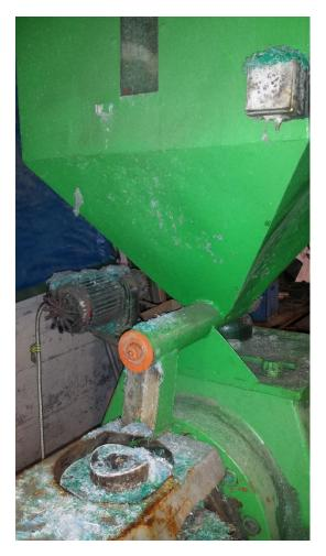
Figure 5 - Feeding system for plastic extruder unit (bis)
