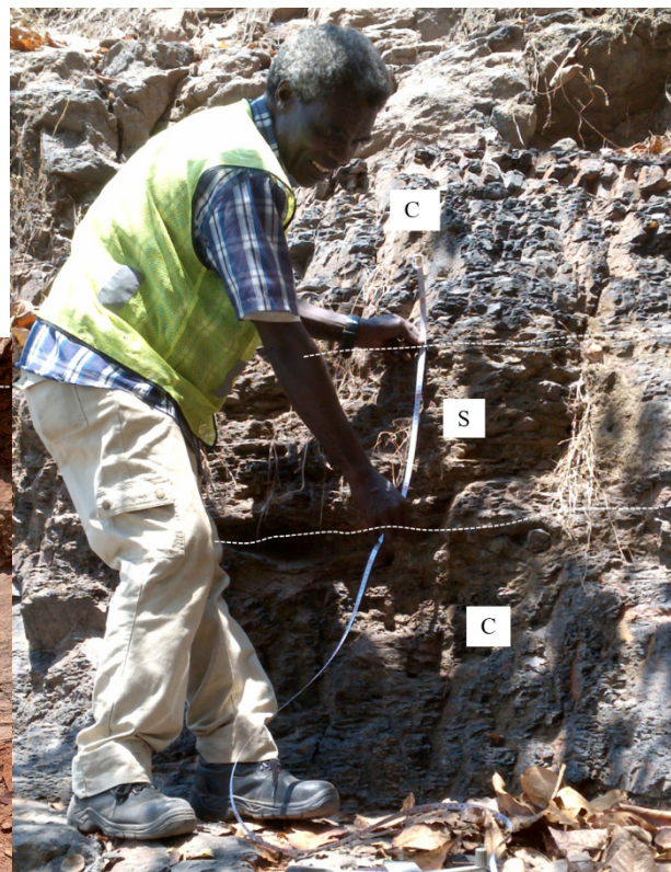
FIGURE 12: Chiweta coal seams (C) and interbedded sandstone arkoses (S) separated by white dotted line
