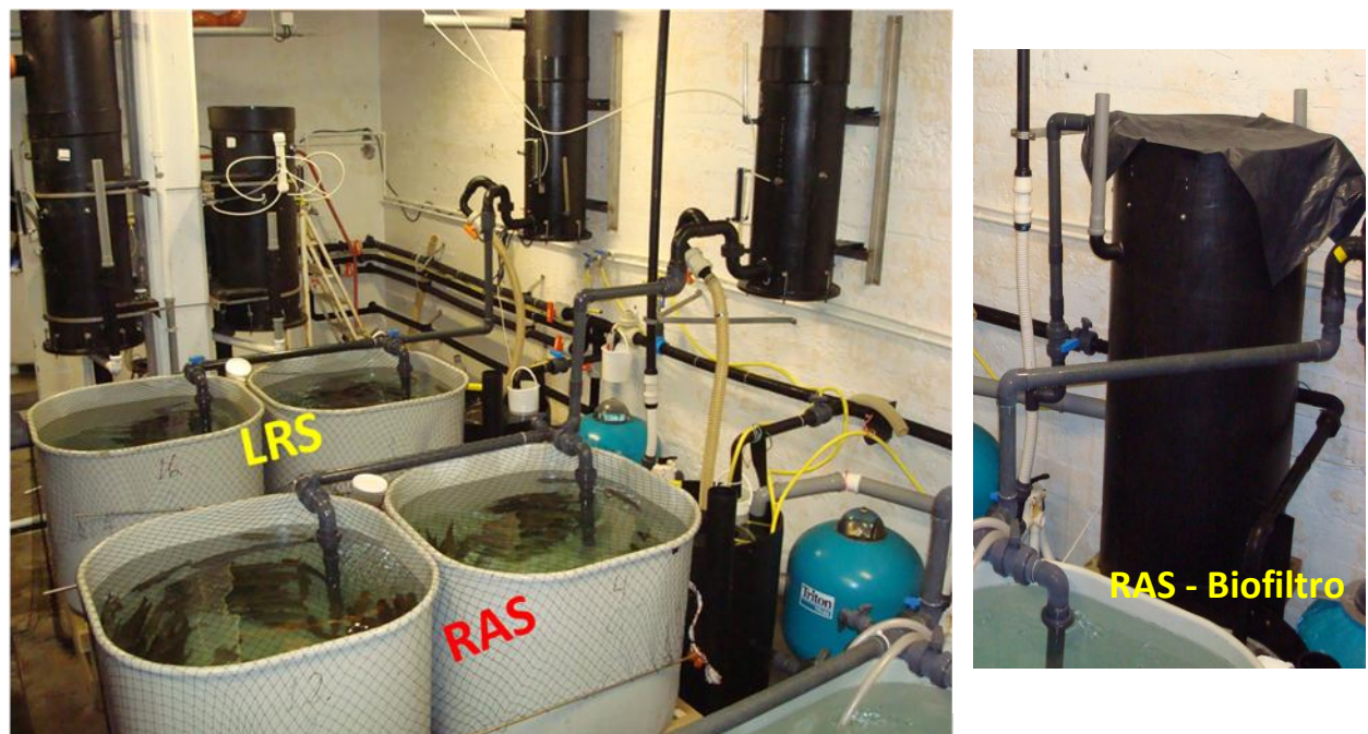
Figure 3: Aquaculture systems used for the experiment. Limited reuse system (LRS) and recirculating aquaculture system (RAS) with biofilter.
