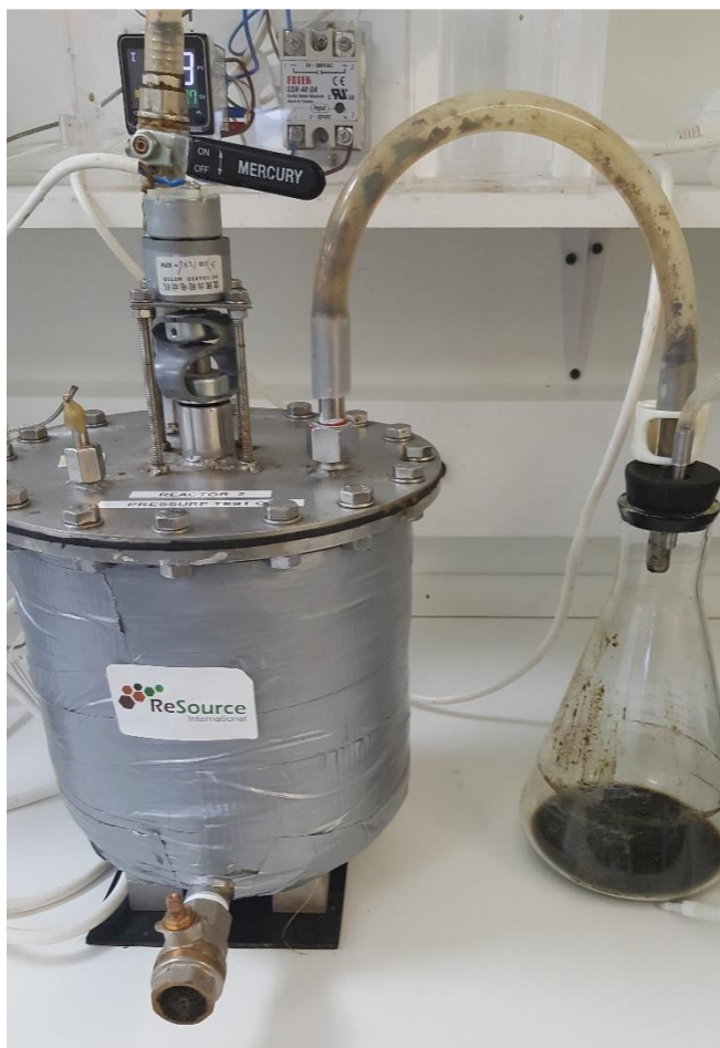
Figure 23 - Biogas reactor. On the right side is the digestate flask used for algae medium (RSI 2016)
