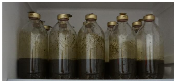
Figure 10: Incubator with the batch test digesters.
