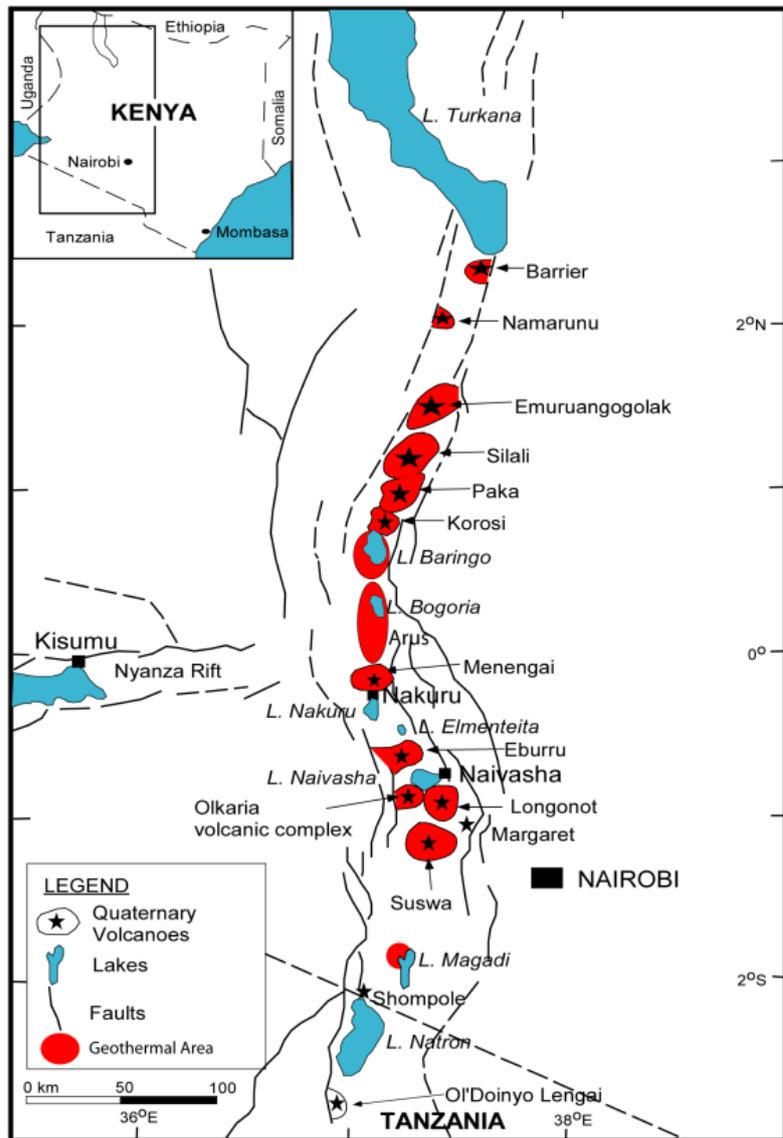
FIGURE 2: Simplified geological map of Kenya showing locations of the geothermal fields and prospects
