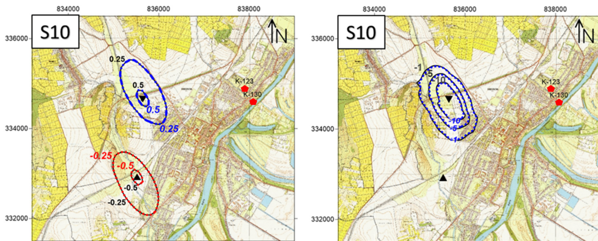
FIGURE 18: Calculated long-term effects of the proposed well duplet on the water level and temperature for Scenario 10
