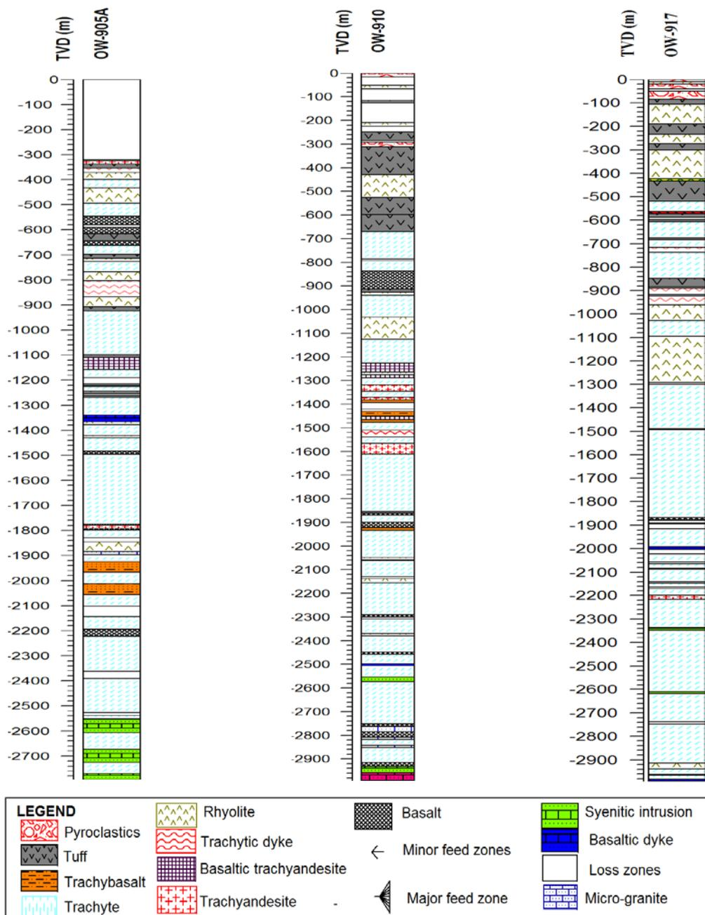
FIGURE 7: The rock units observed in the three wells under the four analytical techniques
