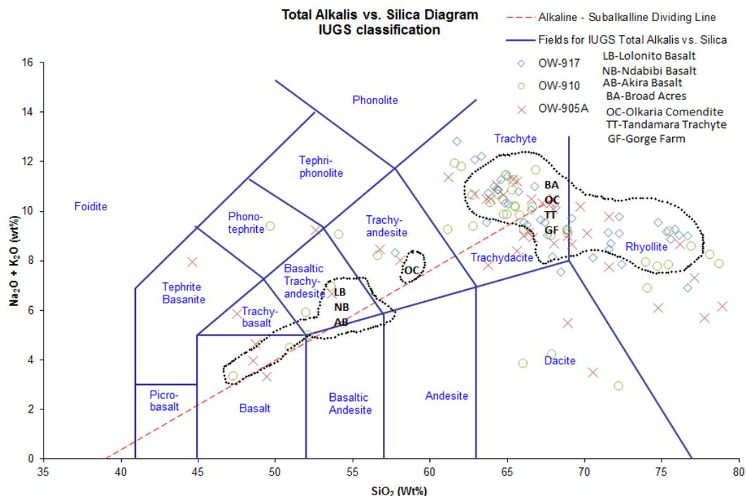
FIGURE 13: TAS classification scheme plot showing the compositional range for the Olkaria sub-surface rocks with the superimposed surface samples data (fields delineated with dotted lines)
