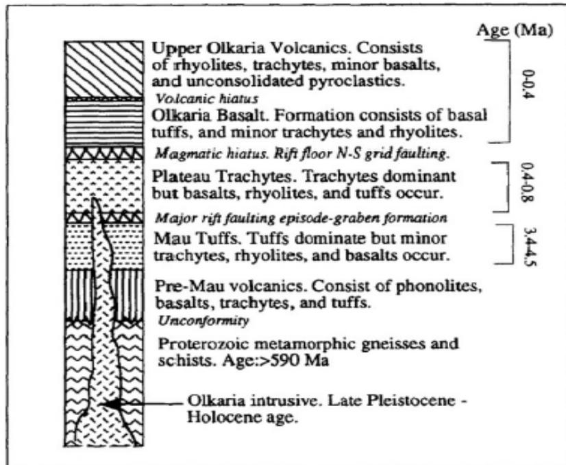
FIGURE 5: Rock units and stratigraphic correlation of drilled wells in Olkaria geothermal area (from Lagat, 2004)
