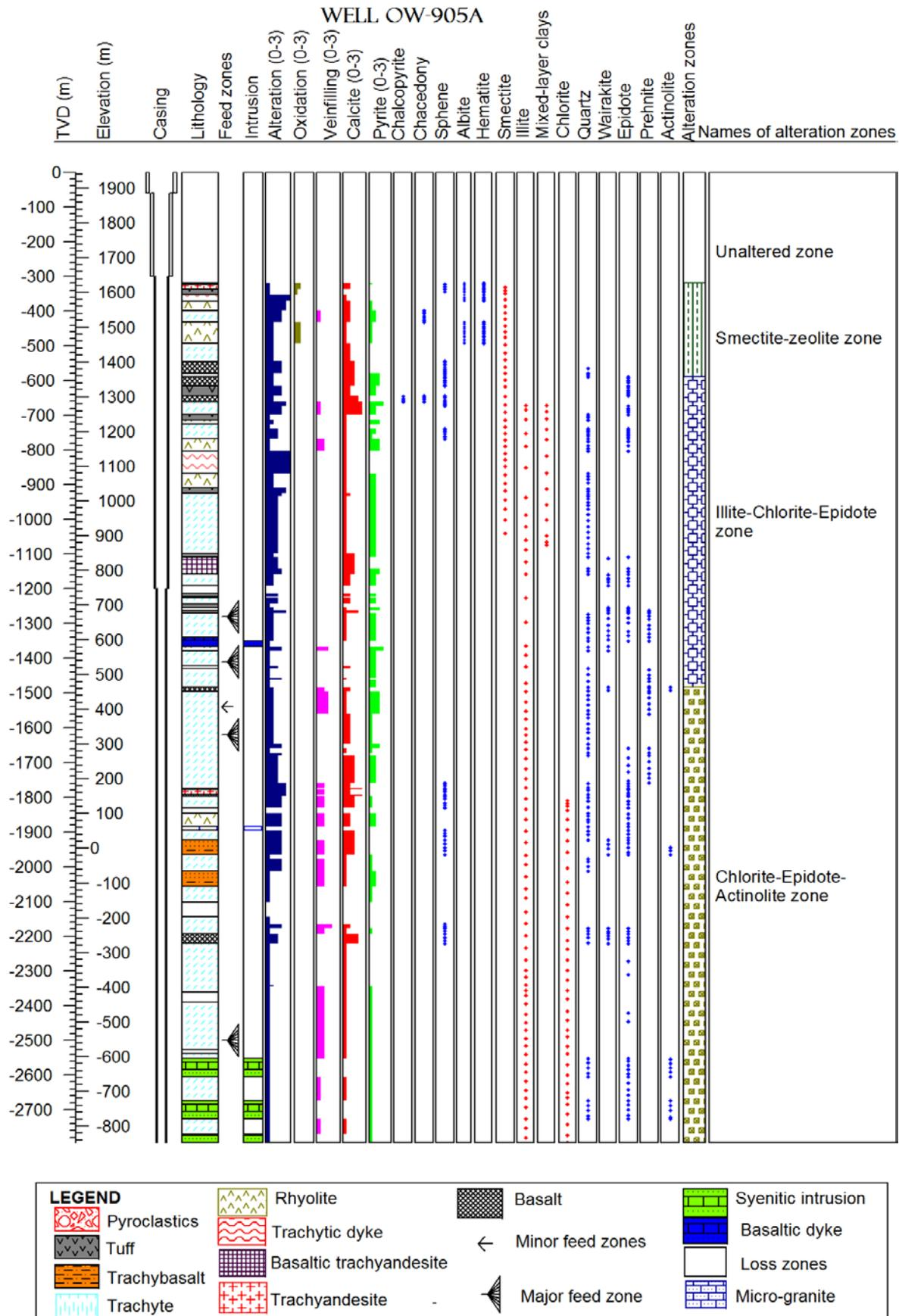
FIGURE 9: Lithology, alteration minerals and alteration zones of OW-905A
