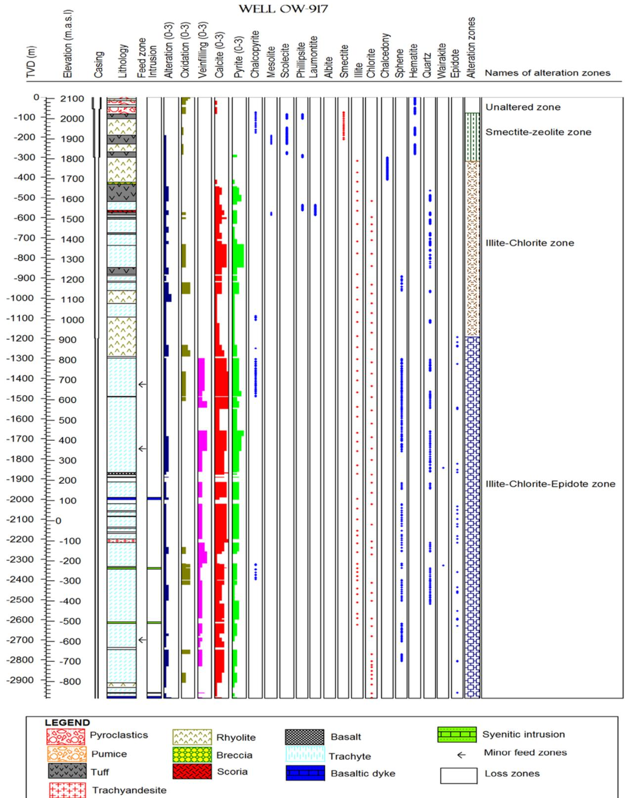
FIGURE 11: Lithology, alteration minerals and alteration zones of OW-917
