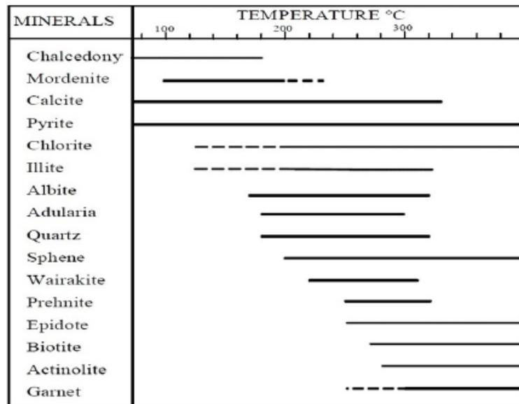
FIGURE 8: Various depositional temperature for different alteration minerals (From Lagat, 2004)
