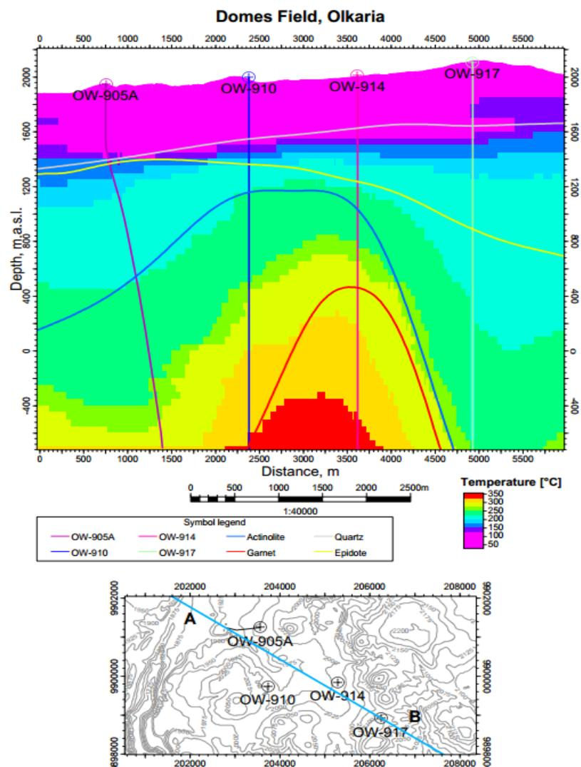
FIGURE 12: Formation temperatures and alteration mineral isograds cross section across AB
