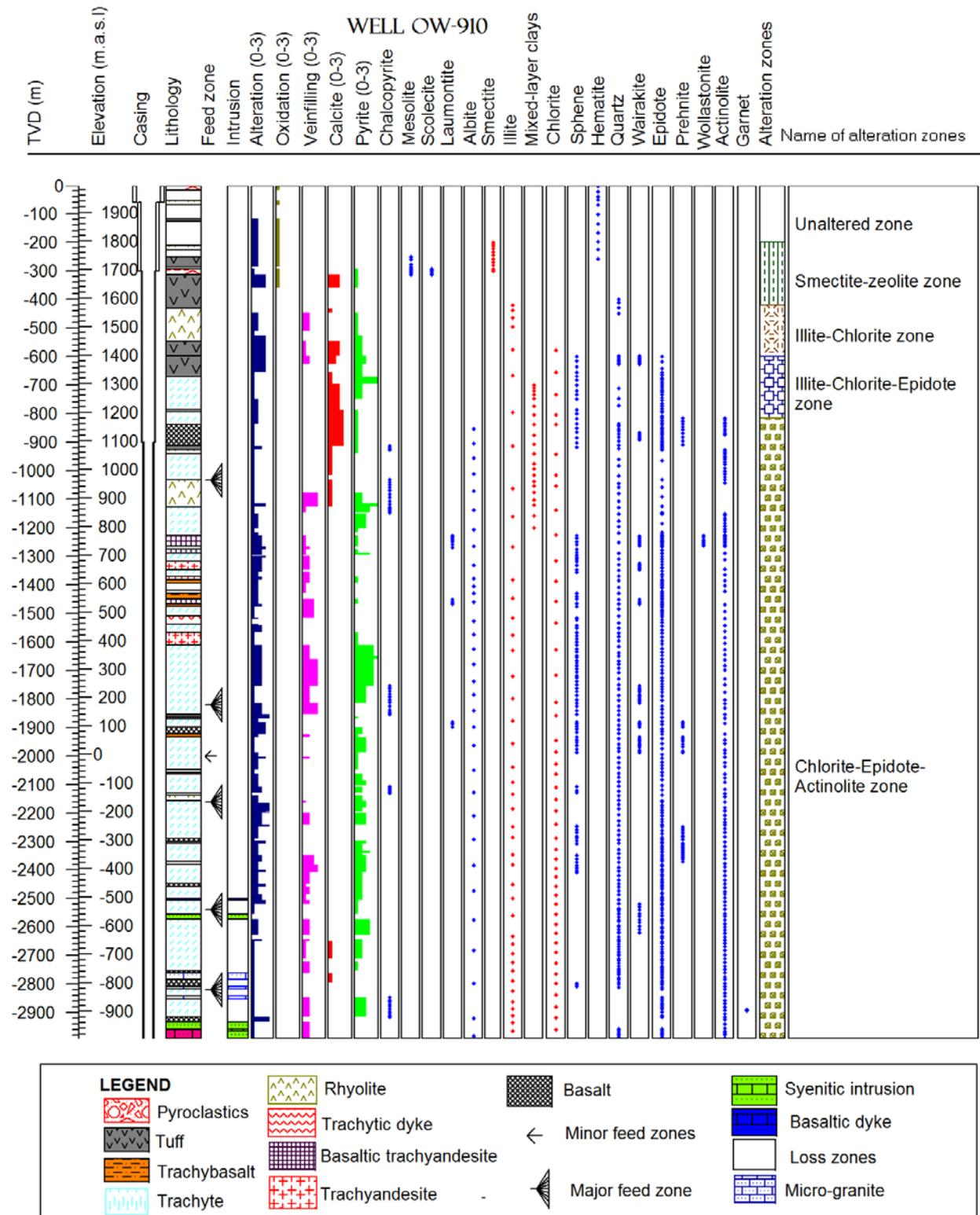
FIGURE 10: Lithology, alteration minerals and alteration zones of OW-910
