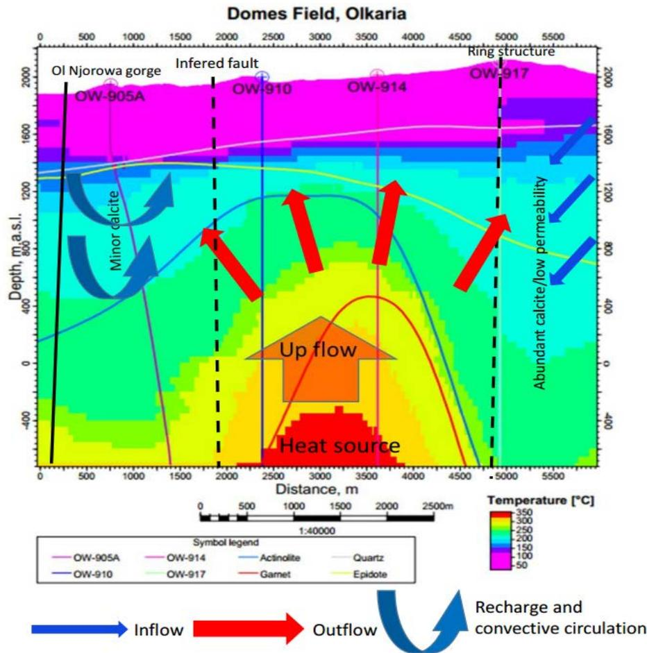
FIGURE 17: Conceptual model of the Domes area based on the research findings of this study
