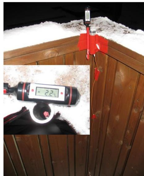
FIGURE 16: Air temperature measurement point
