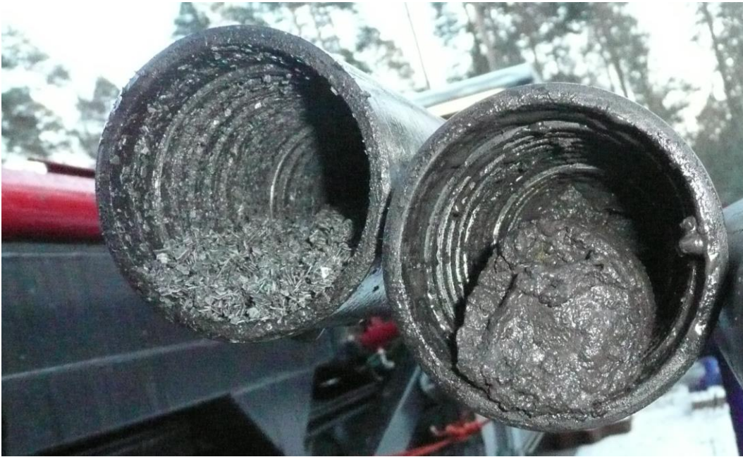
Figure 26 Heavy metal scaling (predominantly native copper, barite, and laurionite) removed from the production well at the geothermal site Groß Schönebeck (2013).
