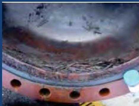
Barite scales from heat exchanger (Scheiber et al., 2014)
