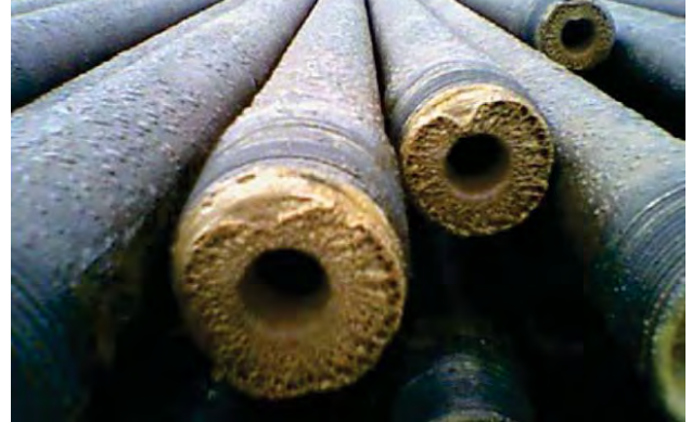
Barium sulphate scaled-up tubing example (Tom Grant and Johnny Smith, Gaither Petroleum, in Jonathan Bellarby, 2009, Well Completion Design)
