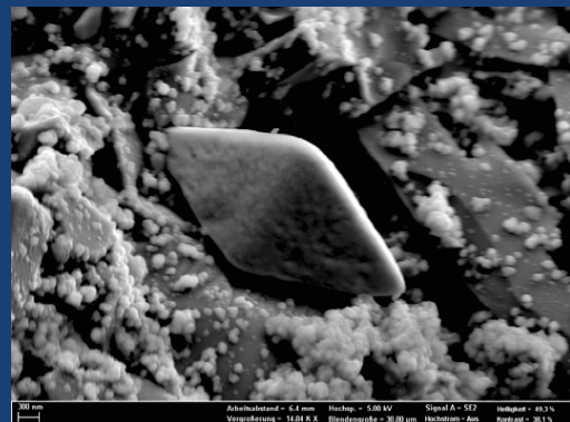
SEM image of scaling (Barite, Laurionite, Magnetite) (Regenspurg, 2013)
