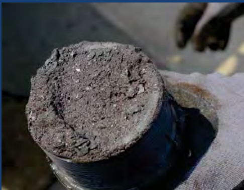
Scalings from a prouction well in the filter area (Regenspurg, 2013)
