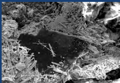
SEM image of scaling (Barite, Laurionite) (Wolfgramm, 2014)
