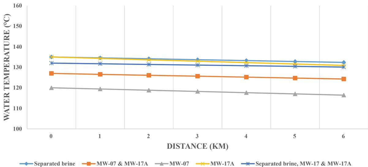
FIGURE 19: Temperature of hot water along a pipeline
