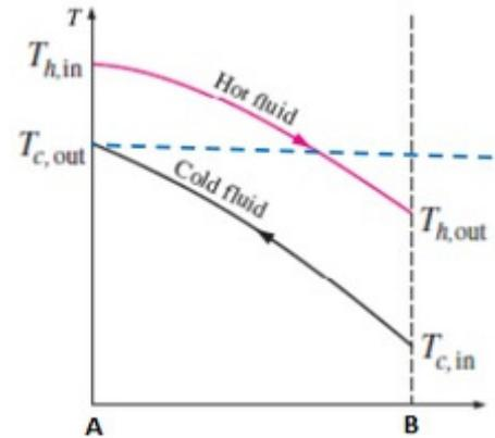
FIGURE 12: Counter current flow temperature profile (Haslego and Polley, 2002)
