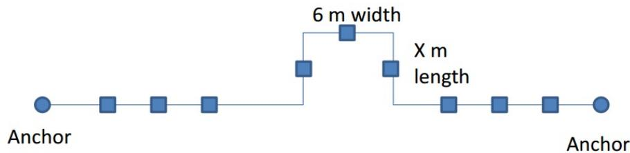
FIGURE 15: Section of a hot water pipeline between two anchors (Harvey, 2015)
