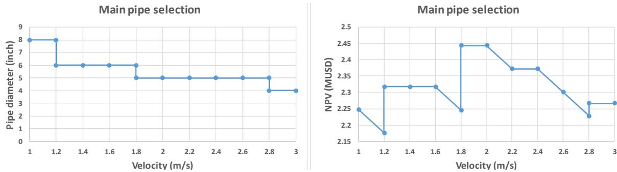
FIGURE 14: Sizing of a water pipeline
