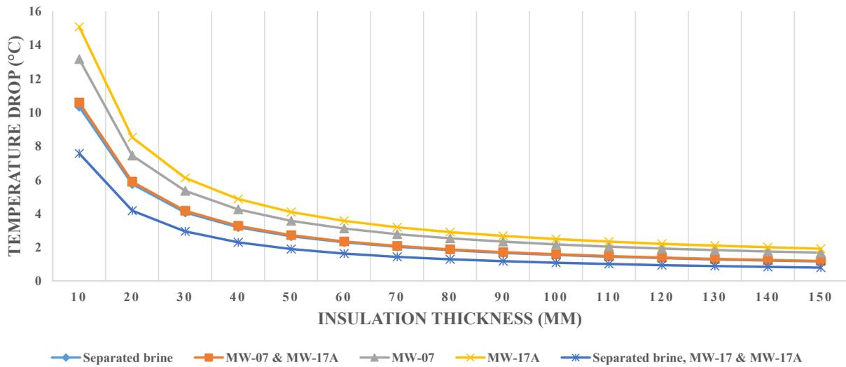
FIGURE 18: Temperature drop as a function of insulation thickness
