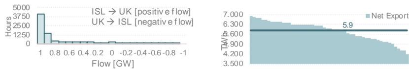
Figure 39: Expected distribution of the hourly level of flow (left) and cumulative net expected exports per scenario, or year, (right) of the IceLink for the Inter-regional transmission expansion option
