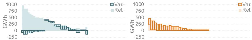
Figure 36: Secondary energy (left) and buyback energy (right) requirement variation with additional demand response with respect to Inter-regional case without wind by 2030<sup>24</sup>
