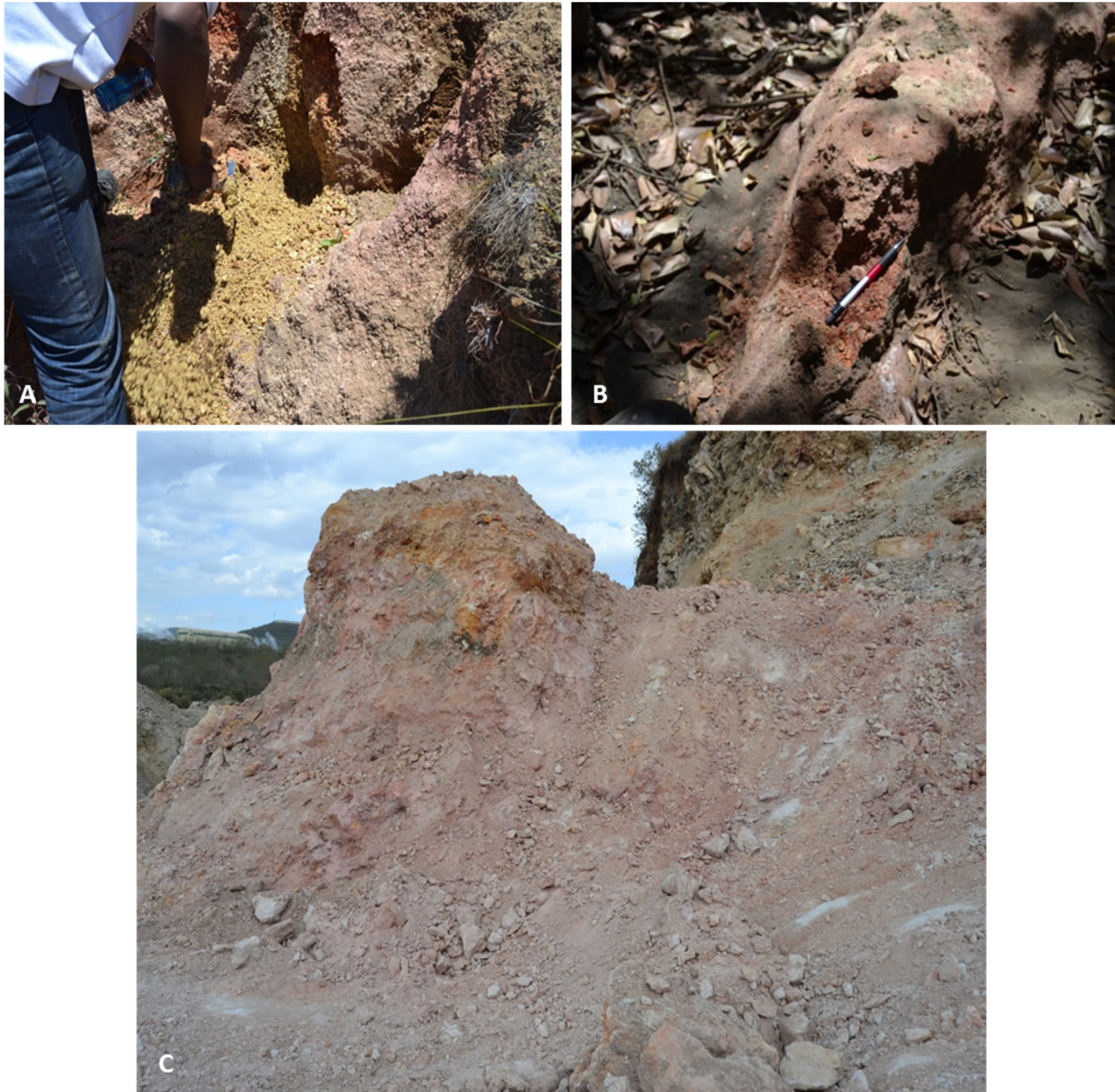
FIGURE 27: Altered grounds showing different levels of alteration. Plate A was taken on altered pyroclastic rock outcrop to the south of Olkaria ring structure where the ground temperatures were 67°C, while in plates B and C, there were no elevated temperatures. The dominant clays were smectite and kaolin altered from pyroclastics and rhyolites
