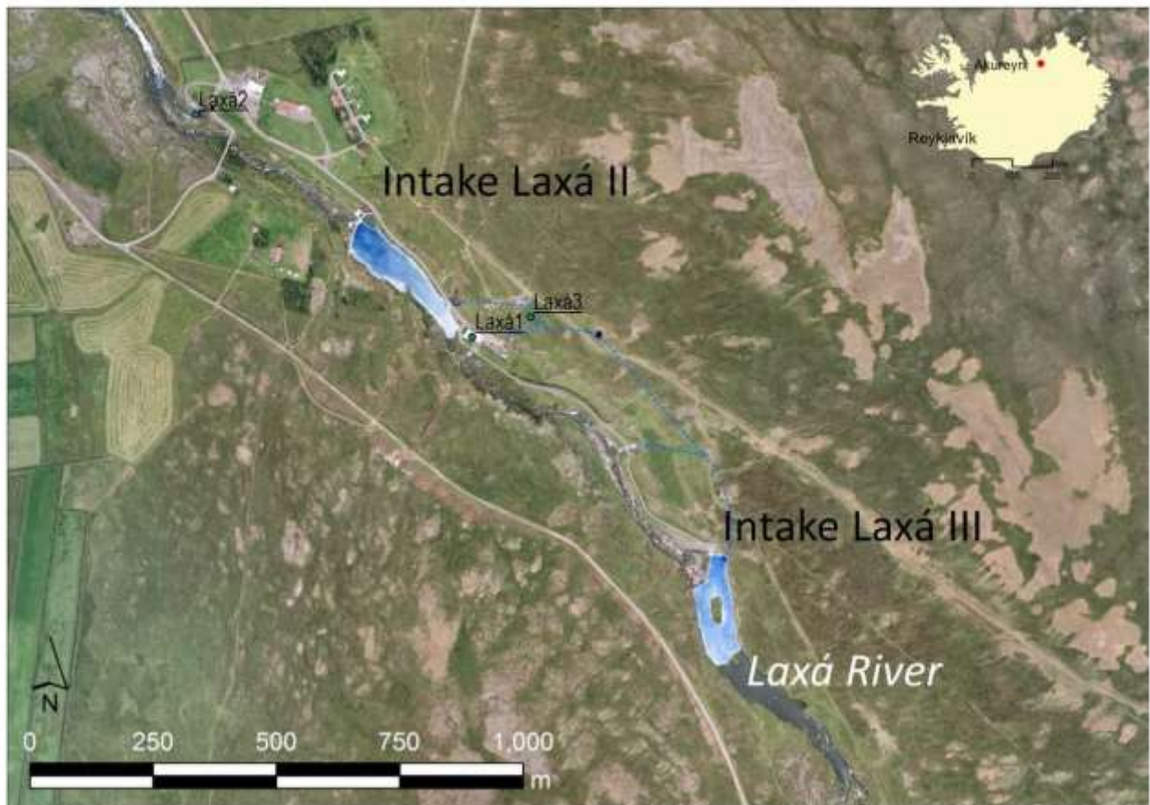
Figure 3 – overview of Laxá II and Laxá III sitting. Blue dotted lines show tunnels from the upstream pond to the downstream.
