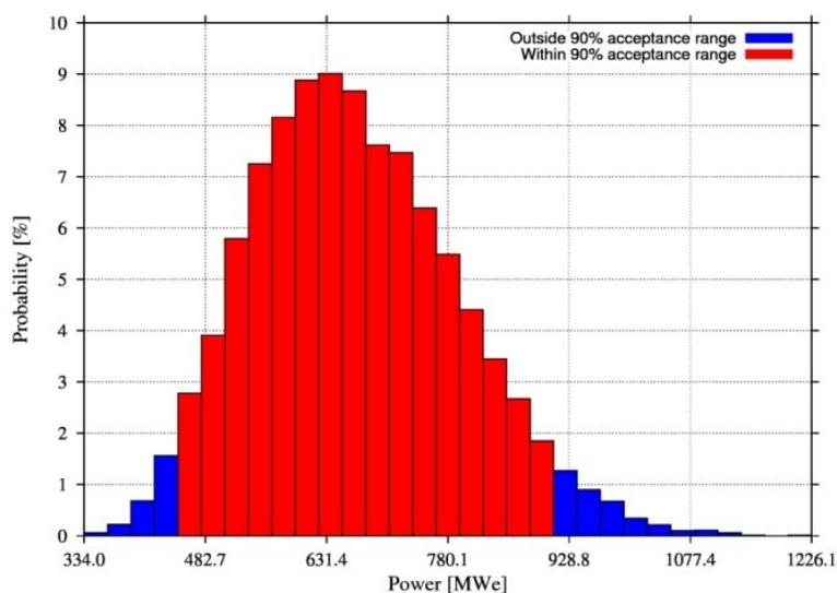
FIGURE 8: An example of the results of a volumetric resource assessment for the so-called “heavily-explored part” of the Olkaria geothermal system in Kenya for a 50-year generation period (Axelsson et al., 2013). The Monte Carlo method was applied in the assessment. Note the great uncertainty in the results (electrical generation capacity) which arises from the uncertainty in key parameters.
