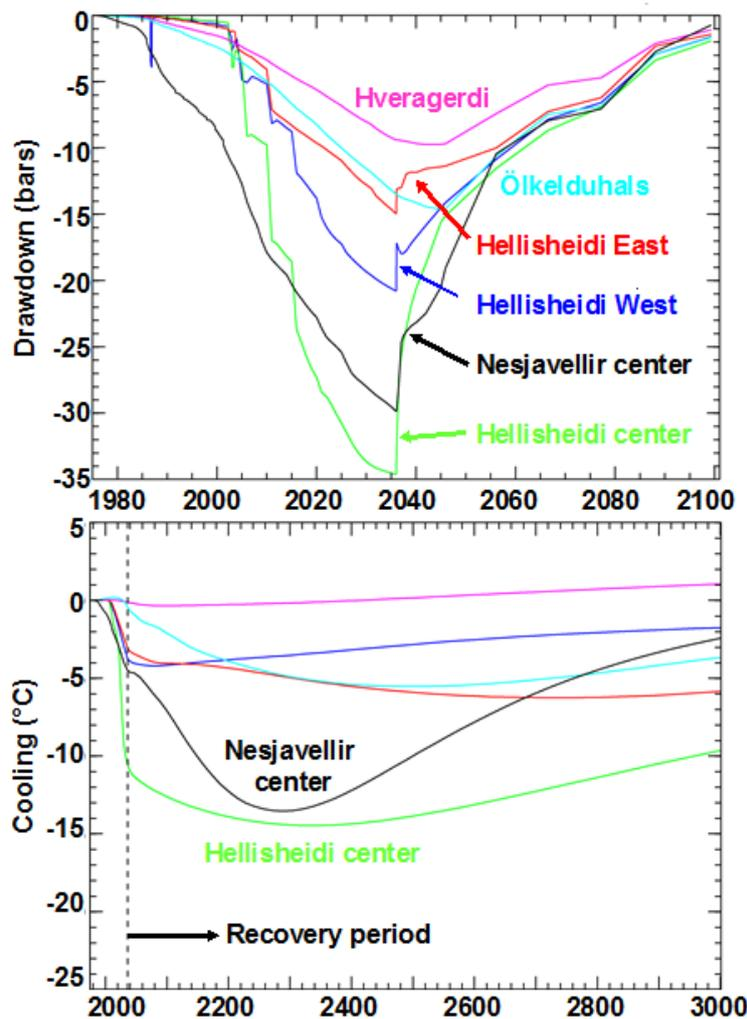
FIGURE 13: Calculated changes in reservoir pressure and temperature in different parts of the Hengill geothermal system in SW-Iceland, during a 30-year period of intense production, and for the following recovery (production stopped in 2036). Note that predicted temperature changes are not well constrained. Figure from Axelsson et al. (2010); see also Björnsson et al. (2003).
