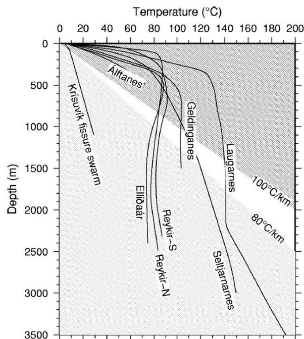
FIGURE 2: Formation temperature profiles for low-temperature systems in and around Reykjavík in SW-Iceland demonstrating the convective nature of the systems, through which heat has been transported from depth up to shallower levels (from Björnsson et al., 2000). Lighter shading denotes temperatures lower than to be expected from the regional gradient and darker shading the opposite.
