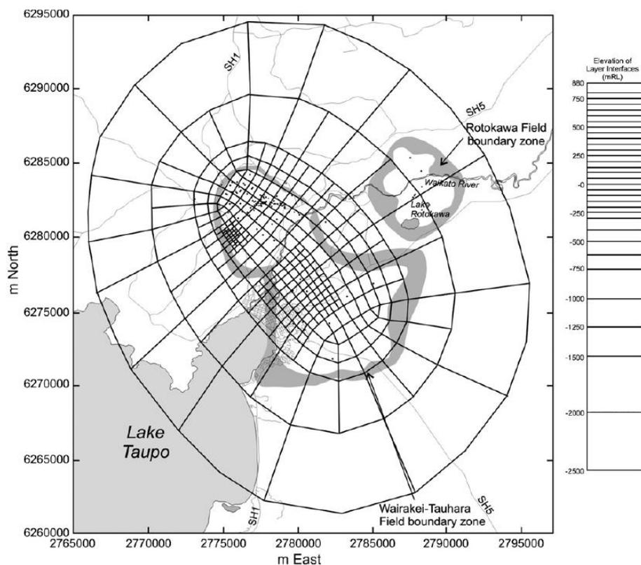
FIGURE 12: A horizontal and vertical sketch of the computational grid a recent numerical reservoir model of the Wairakei geothermal system in New Zealand (O'Sullivan et al., 2009)
