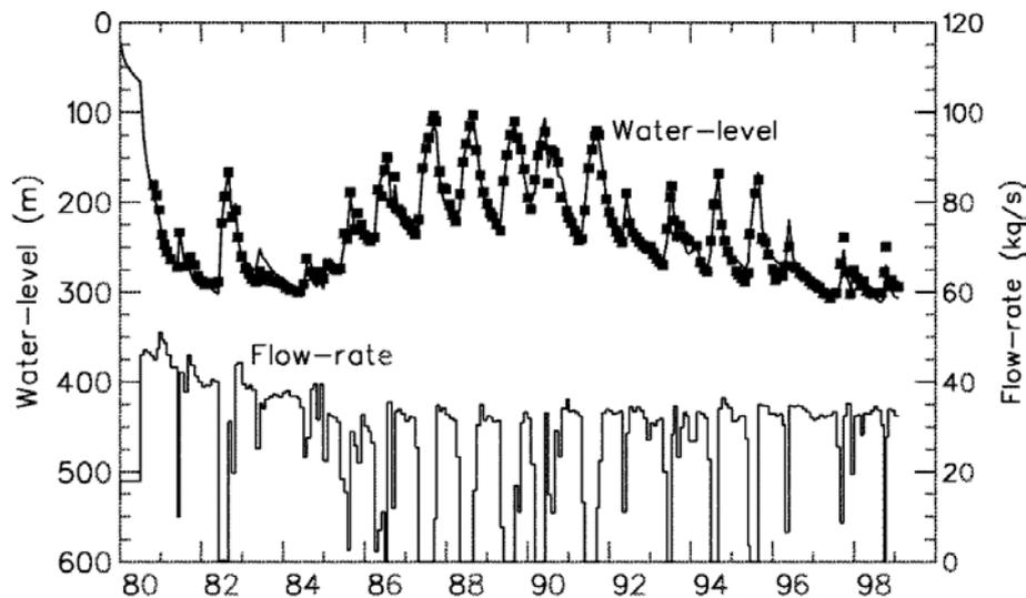
FIGURE 10: Production and water level history of the Ytri-Tjarnir low-temperature geothermal system in central N-Iceland 1980-1999. The water level history has been simulated by a lumped parameter model (squares = observed data, line = simulated data; Axelsson et al., 2005).
