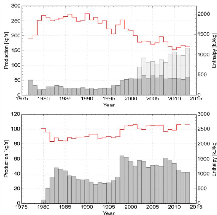
FIGURE 7: Production and enthalpy discharge histories of two sub-areas of the Krafla volcanic geothermal field in NE-Iceland (from Weisenberger et al., 2015). The upper half shows declining enthalpy due to colder recharge (inflow) and reinjection (pressure support reduces boiling) while the lower half shows increasing enthalpy due to increased boiling.
