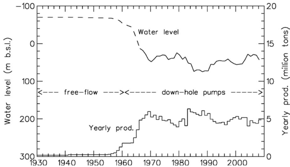
FIGURE 4: History of production and water level (pressure) response of the Laugarnes convective geothermal system in SW-Iceland from 1930 (Axelsson, 2012)
