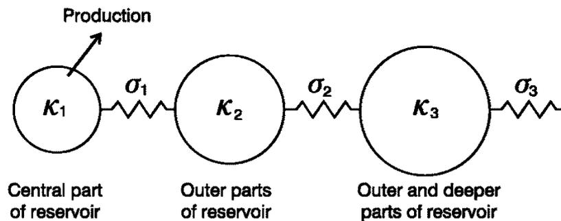
FIGURE 9: A 3-tank lumped ladder model commonly used to simulate geothermal systems (Axelsson et al., 2005)
