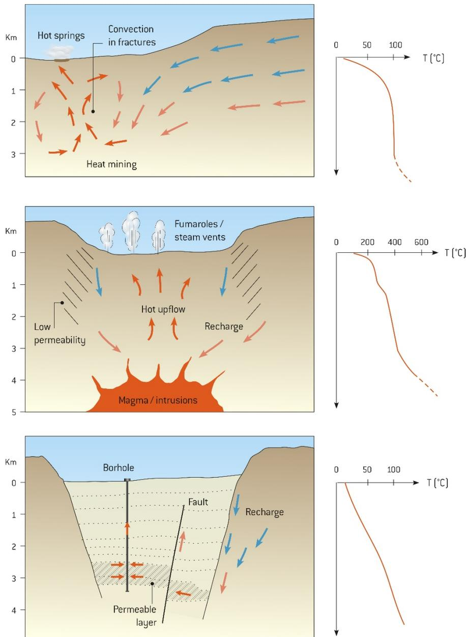
FIGURE 1: Schematic figures of the three main types of geothermal systems (A, B and C) along with typical temperature profiles
