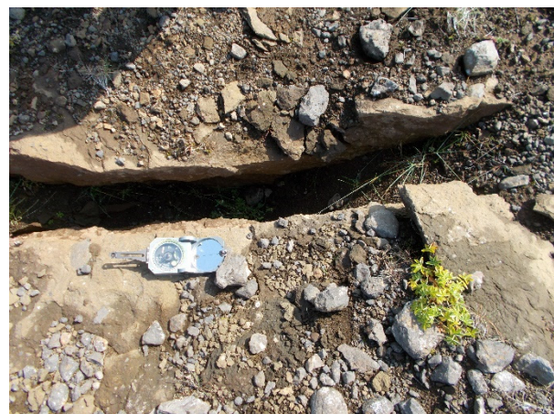
FIGURE 8: Fracture direction N 30°E with around 13 cm opening
