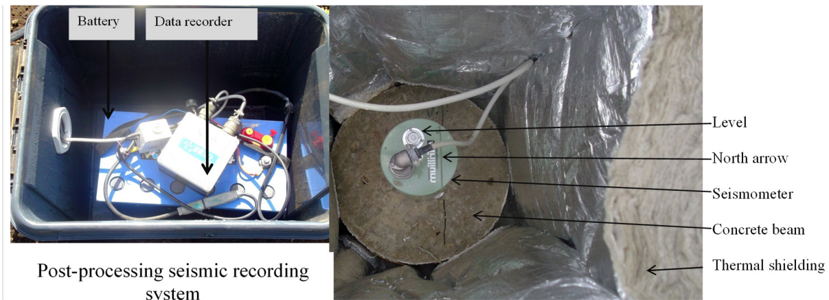
FIGURE 10: Parts of the seismic monitoring stations
