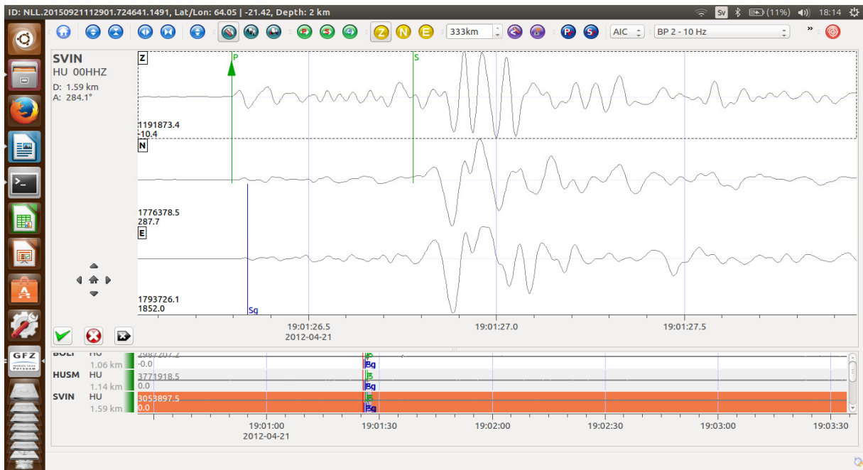
FIGURE 13: Picker window in the SeisComP3 software showing P and S waves from an event in Hellisheidi
