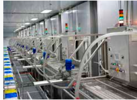
Plate freezers at Sildarvinnslan in East-Iceland. Each unit with 70-80 tn/24 hour capacity.
