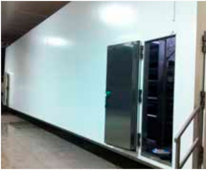
IQF Freezer, 3-4,000 kg/hour for tilapia production at Regal Springs in Mexico.
