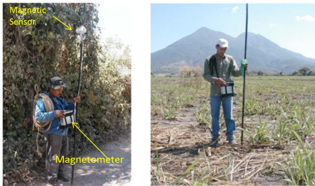
FIGURE 6: Examples of a field measurement with a magnetometer model GEM-19T from GEM System, owned by LaGeo; a magnetic survey in the San Vicente volcano area.
