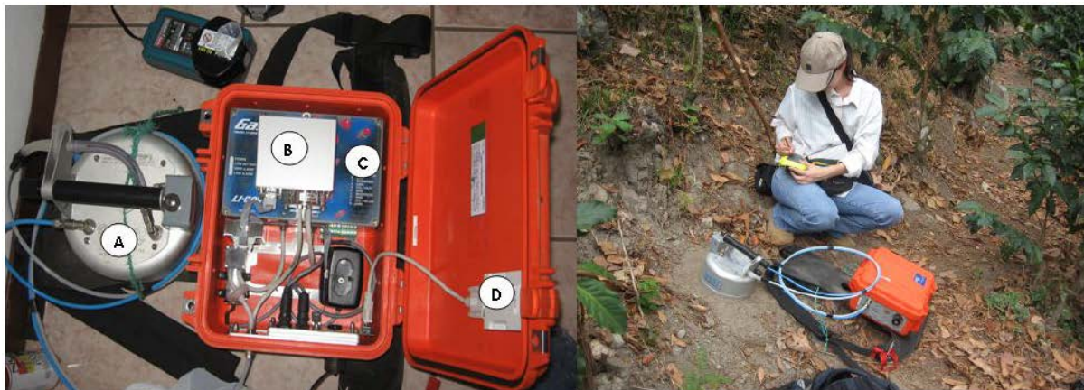
FIGURE 2: Portable diffuse flux meter (Carbon dioxide and Hydrogen sulfide) set up for determination of flux in soil (Gutiérrez, 2009)
