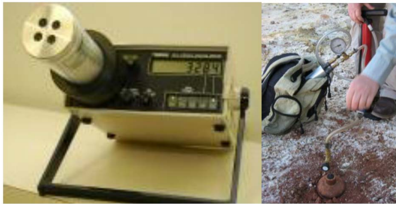
FIGURE 1: Pylon portable radiation monitor set up for determination of radon in soil (Grimaldi, 2010)
