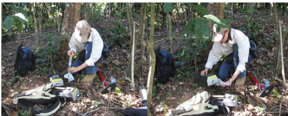
FIGURE 3: Set up for mercury vapour and Hydrogen sulfide analyzer (Gutiérrez, 2009)
