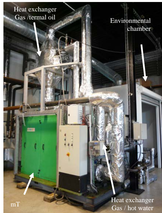
Figure 3: Trigeneration system in the CREVER-URV test bench
