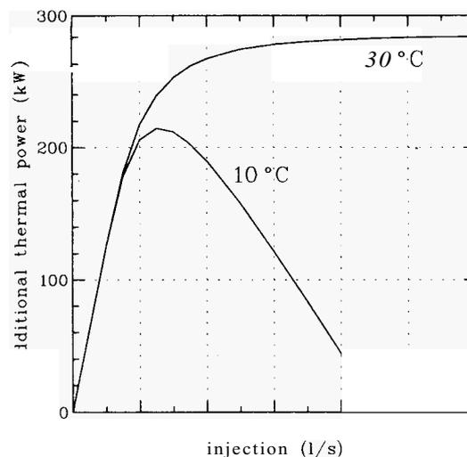
Figure 11. Calculated additional thermal power resulting from injection into well 6 at Thelamork of 10 and 30 °C water respectively.
