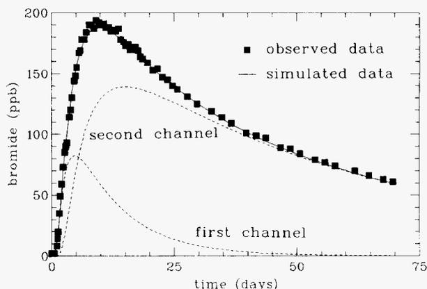
Figure 6. Observed and simulated bromide recovery curves for the well dipole 6-11 at Thelamork.
