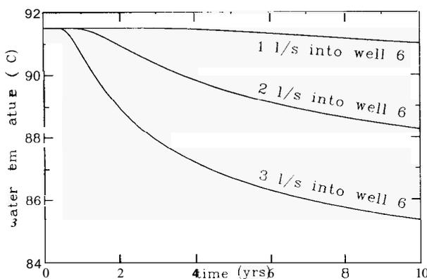
Figure 10. Calculated cooling of water from well 11 at Thelamork due to reinjection of 30 °C water into well 6.
