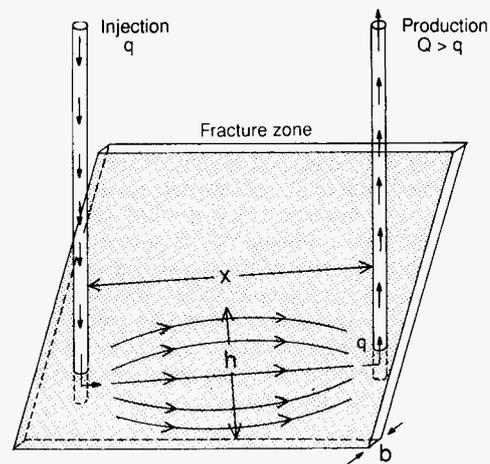
Figure 5. A simple model of a fracture-zone connecting a reinjection-production well dipole.
