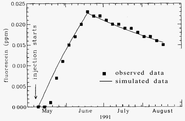
Figure 8. Observed and simulated fluorescein recovery at Laugaland. Water is injected for the first 40 days.
