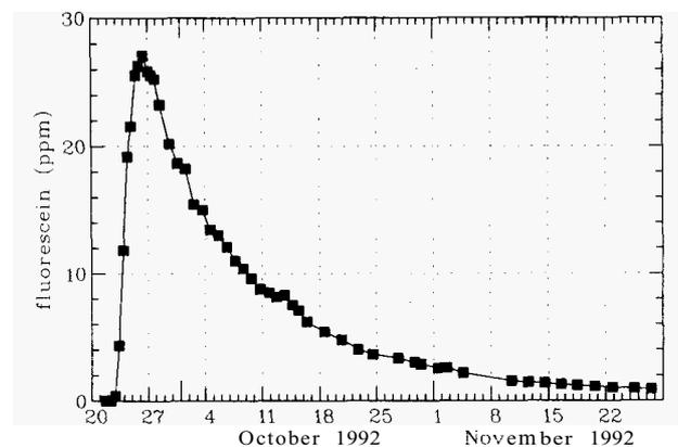
**Figure 3. Observed fluorescein recovery in well 8 at Urriðavati during a tracer test.**
