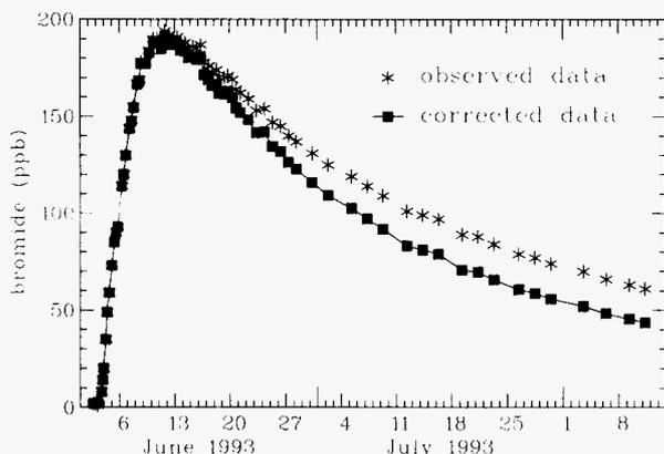
Figure 4. Observed and corrected bromide recovery curves for the well dipole 6-11 at Thelamork.
