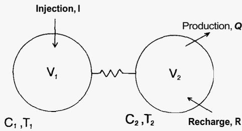
Figure 7. A simple lumped model used to simulate the tracer return during the Laugaland experiment.
