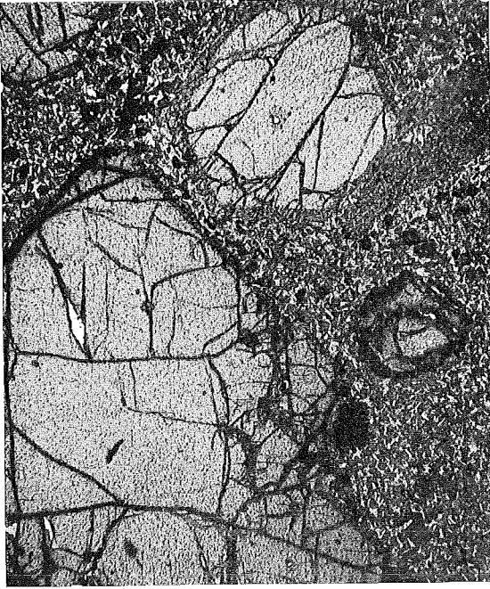
Pl. III a. Mantled olivine and pyroxene phenocrysts in granular groundmass. The rim of the olivine is emphasized by the selective alternation of the second phase of crystallization (mantle and groundmass crystals). Plane polarized light x 15.
