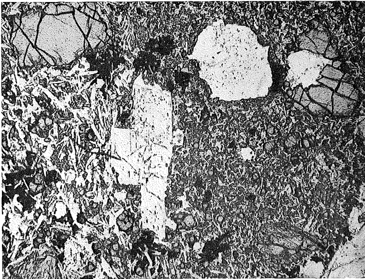
Pl. V b. Photomicrograph to illustrate two types of texture occurring together without any signs of intrusive relationships between the two. The plagioclase phenocryst contains inclusions of magnetite. Plane polarized light x 15.
