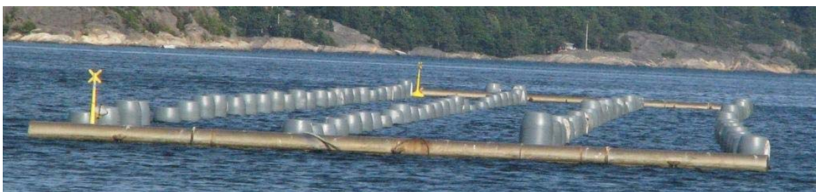
Picture 5 Rig with 10m stainless steel tube frame each end with 4 lines 120m long
