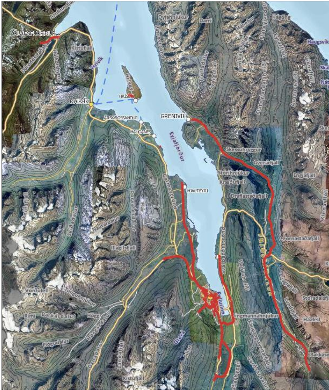
Figure 76. The district heating services of Norðurorka in Eyjafjörður. The red lines show extent of pipelines for hot water (Norðurorka, Webpage b).
