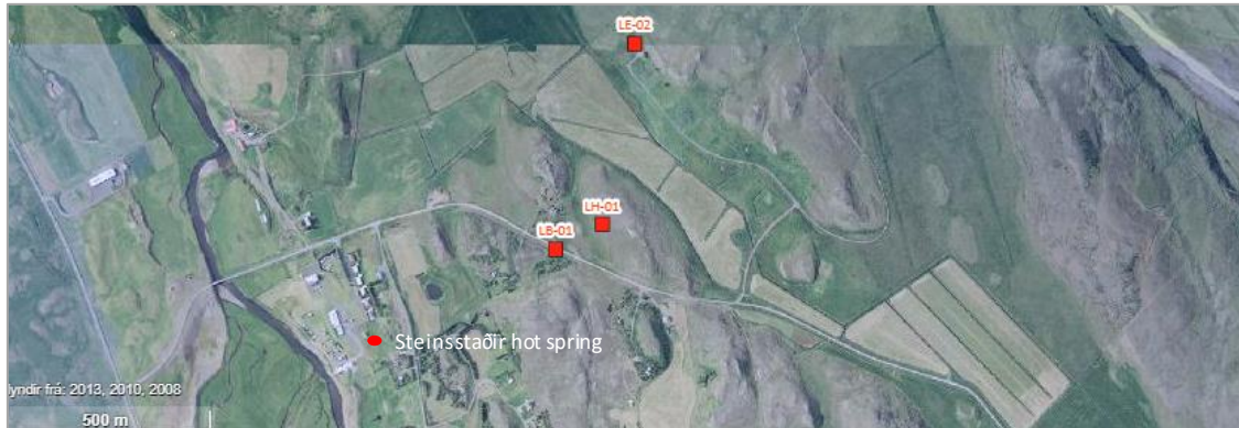
Figure 57. Overview of the production wells and the hot spring in the Steinsstaðir well field (modified from NEA's Geoportál).
