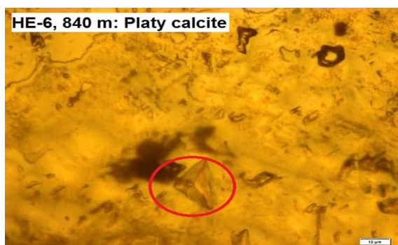
FIGURE 8: Secondary fluid inclusion from fracture fillings of platy calcite in the mixed layer clay-chlorite zone at 840 m
